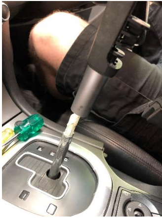
5. Pull the original shifter body off the shaft
