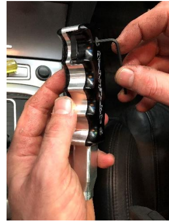
6. On your new RipShift, undo both side cover panels with supplied Allen key (2.5mm)
